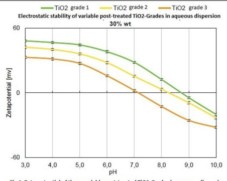
Fig.1: Zeta-potential of three variable post-treated TiO2-Grades in aqueous dispersion with a concentration of 30 wt%. Measured with method of Electrokinetic-Sonic-Amplitude ESA.
